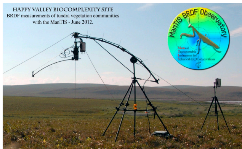
Figure 7. The ManTIS field portable spectro-goniometer of the AWI. This transportable, field goniometer is the first of its kind and is adapted for use in Arctic field conditions. Picture by M. Buchhorn.
