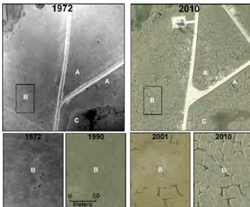
Fig. 3 Changes between 1972 and 2010 near the main road junction in map B. Note changes in infrastructure, including small new gravel pad and building near the top of the photo, a new pipeline and gravel road on the upper right side, and an expanded road intersection. Also note extensive changes in the character of the ice wedge polygons with many more flooded ice wedge troughs between polygons in 2010. Areas near A and B have extensive ice wedge polygons. Numerous scattered small thermokarst pits (small dark ponds) are visible near A in 1972, with little change in 1990. Areas A and B show marked increases in thermokarst in 2001 and even more by 2010. Area C is in a drained thaw lake basin with ice poor soils and shows little evidence of new thermokarst. Changes in area A were mapped as infrastructure related because of the proximity of the road and the pipeline that have significantly altered the hydrology of this area. Area B is not clearly affected by infrastructure.
