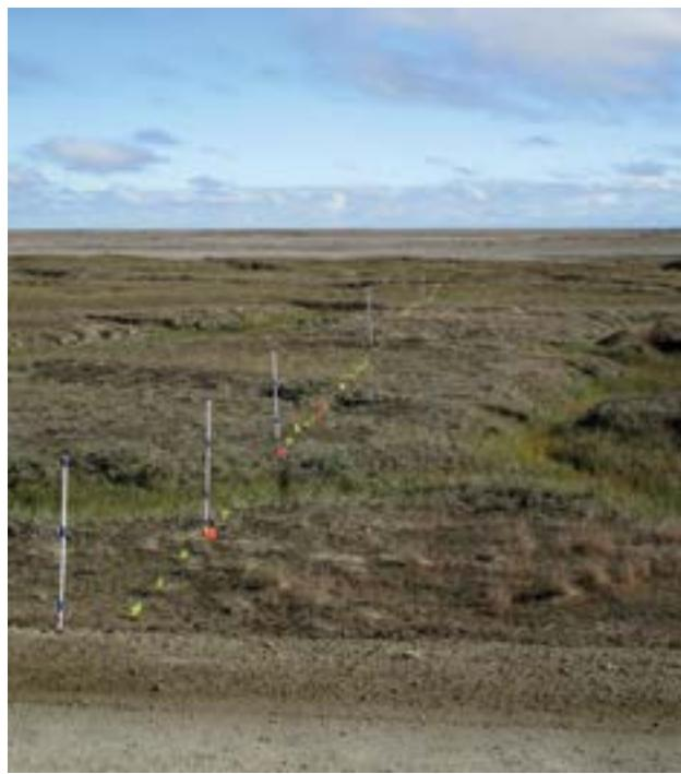
**Figure 1.3.** Transect 3, showing generally dry vegetation and high-centered polygons with  $>0.5$  m of topographic relief. Vertical stakes are at 0, 5, 10, 25, 50 and 100 m. *IMG\_0026.jpg*.
