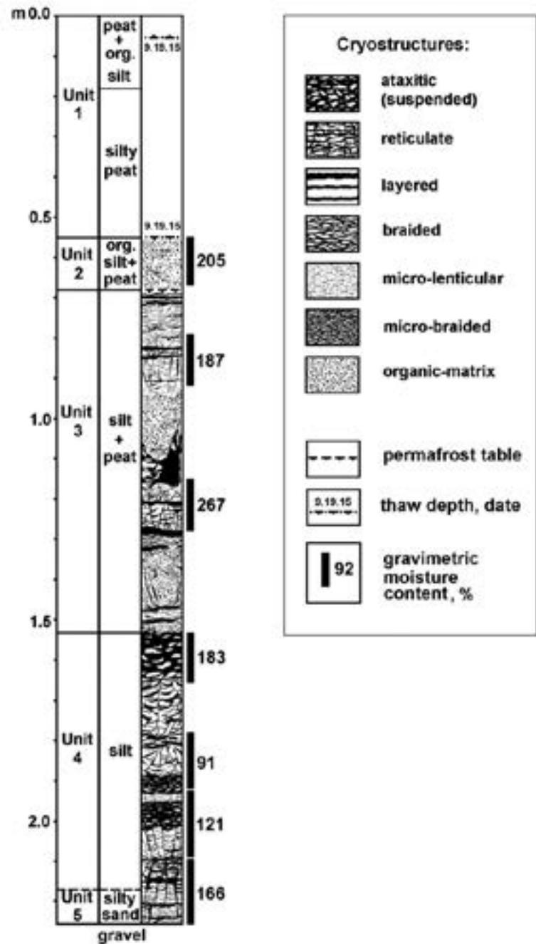
Figure 2.16. Cryostratigraphy of the upper permafrost, Site SR-1, based on borehole drilled in ice-wedge-polygon center (ice is black).
