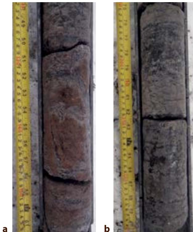
Figure 2.15. Frozen core obtained from borehole SR-1. (a) Ice-rich silt with peat inclusions, 123–154 cm. (b) Ice-rich organic-poor silt, 192–217 cm; ice-rich silty sand with coarse inclusions 217–226 cm.
