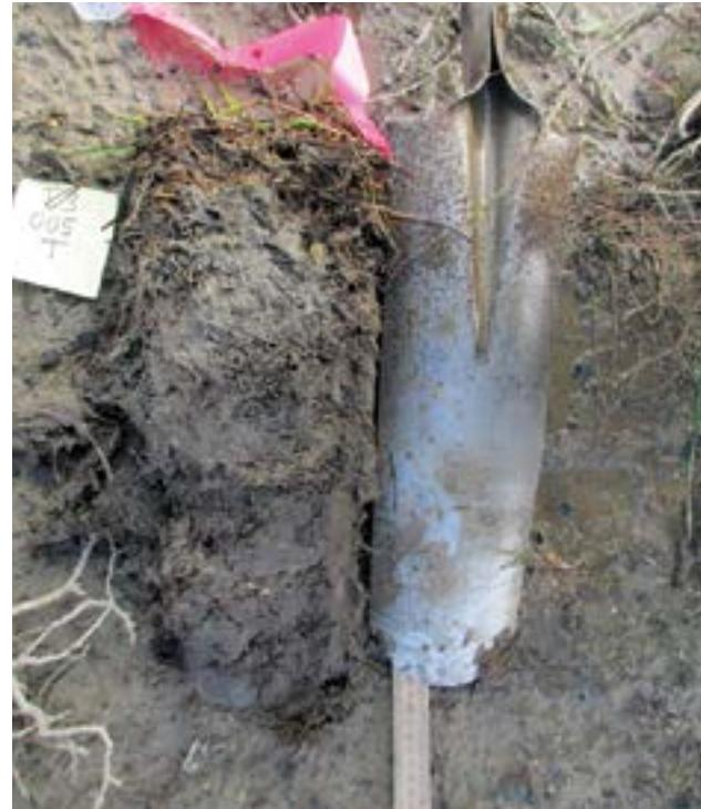
**Figure 2.4.** Soil plug from trough of an ice-wedge polygon 5 m from the road on Transect 3. The back of the Sharpshooter shovel used to extract the soil plugs is shown. Note the gray color at the top of the organic soil horizon underlying the surface layer of moss, indicating leaching of dust into the organic layer. Photo: IMG\_216.
