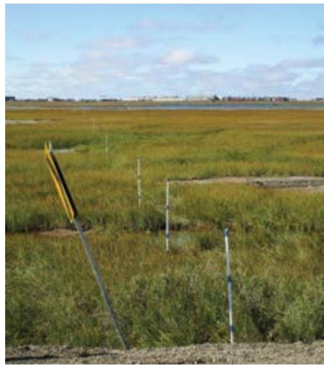
**Figure 1.4.** Transect 4, showing wet tundra with considerable flooding due to blockage of drainage by the Dalton Highway. Vertical stakes at same intervals as Transect 3. *IMG\_0024.jpg*.
