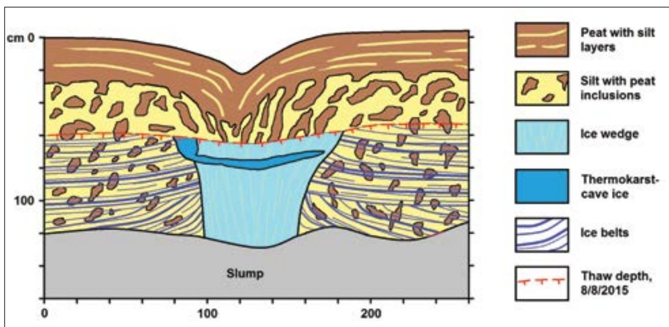
**Figure 2.20.** Cryostratigraphic profile across ice wedge exposed at Site SR-1, August 8, 2015.
