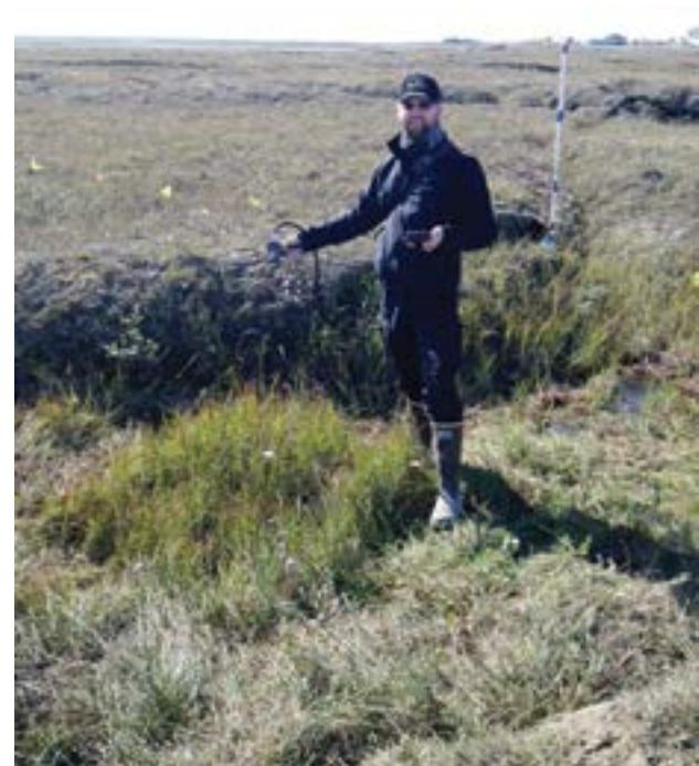
**Figure 2.7.** Marcel Buchhorn measures surface reflectance via field spectroscopy at a permanent vegetation plot in August 2015. Surface reflectance was measured at every 1 m flag and at each permanent plot on the 100-m transects T3 and T4 at the Airport Site.
