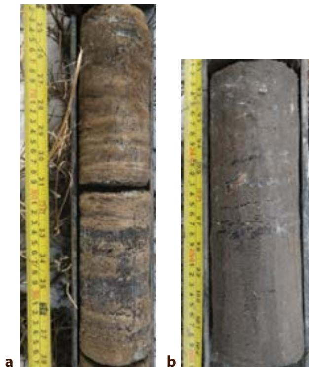
**Figure 2.12.** Frozen cores obtained from boreholes drilled in ice-wedge-polygon centers. (a) Borehole T3-59.0-C, ice-rich organic silt with peat inclusions, 62–97 cm. (b) Borehole T5-65.4-C, ice-rich organic silt, 233–257 cm.
