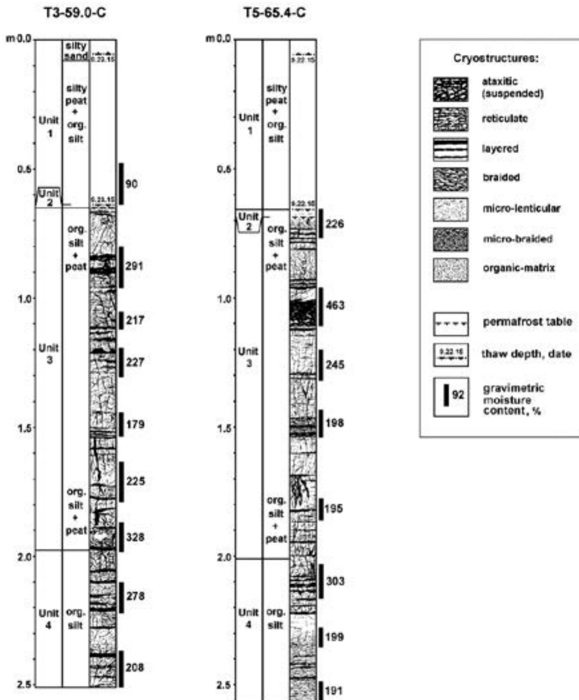
**Figure 2.11.** Cryostratigraphy of the upper permafrost, based on boreholes drilled in ice-wedge-polygon centers (ice is black).
