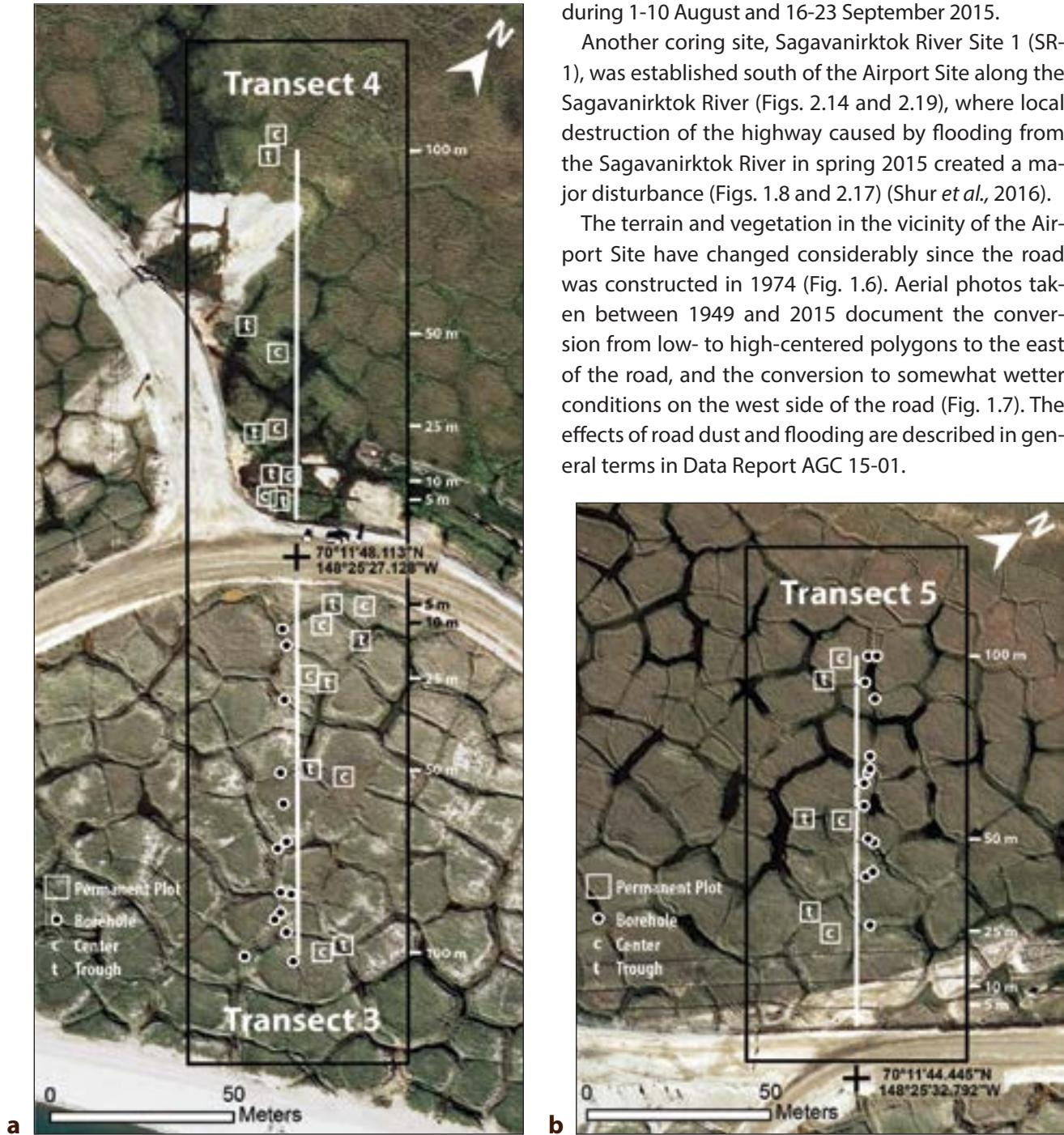
**Figure 1.2.** The Airport Site showing the locations of (a) Transects 3 and 4, and (b) Transect 5. The mostly dry thermokarst terrain with high-centered polygons with >0.5 m of topographic relief along Transect 3 contrasts with the wetter terrain along Transect 4. Transect 5 was established to provide better permafrost coring opportunities west of the road.
