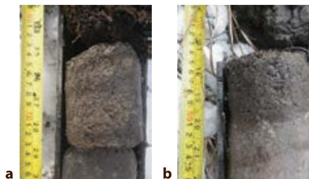
**Figure 2.13.** Photos of the intermediate layer (IL) above ice wedges in boreholes drilled on T3 and T5. (a) Borehole T3-100.7-T, 59–76 cm (IL - 62–72 cm). (b) Borehole T5-88.3-T, 38–57 cm (IL - 46–51 cm).
