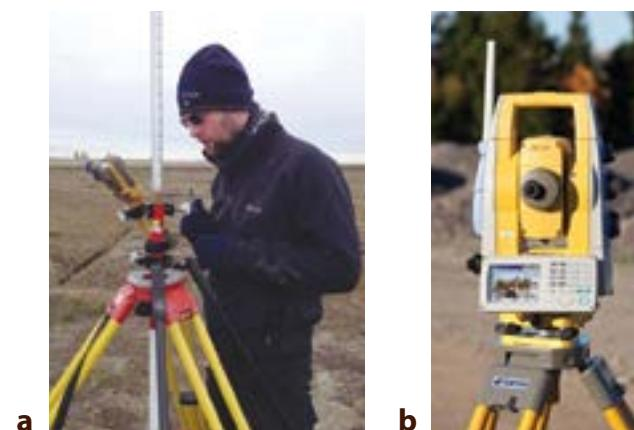
**Figure 2.5. (a)** Marcel Buchhorn surveying plot markers using a Topcon RTK GPS HyPer Lite + GPS system. **(b)** Topcon IS-3 Imaging Station and Laser Scanner. Photo: Topcon.
