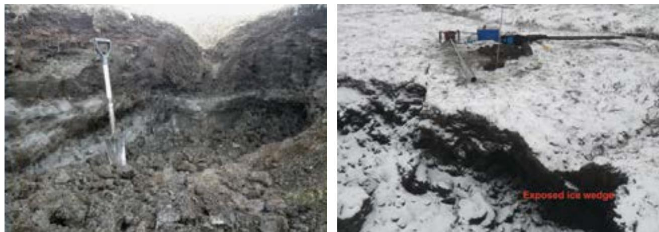
**Figure 2.18.** Ice wedge exposed at Site SR-1, August 8, 2015. This exposure is also shown in the drawing in Fig. 2.20.
