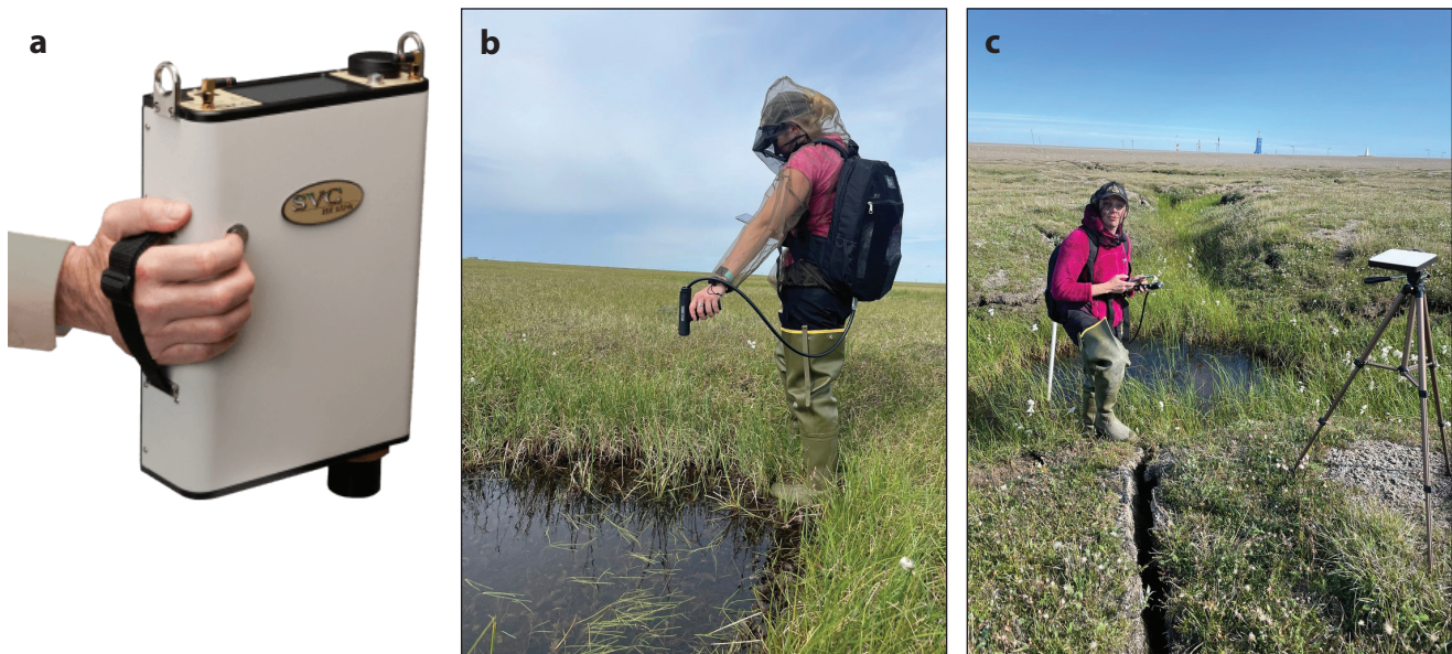
Figure 8. a. Spectra Vista Corporation (SVC) field-portable spectroradiometer, model HR-1024i. b and c. Kelcy Kent making field measurement of NDVI with the spectrometer carried in a backpack linked and a fiber-optic cable to a hand-held 25° field of view radiation sensor. Note in c the reflective calibration whiteboard mounted nearby on a tripod. Credits: a, Courtesy of Spectra Vision Corp.; b and c, Amy Breen.
