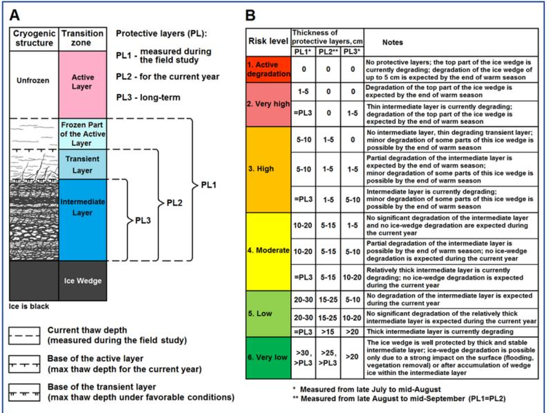
**Figure 4.** Estimation of risk of the ice-wedge degradation. A – Protective layers of frozen soils preventing wedge ice from thawing; B – Evaluation of risk of the ice-wedge degradation for northern Alaska.
