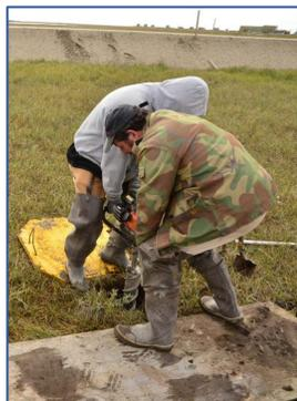
**Figure 5.** Permafrost drilling with the SIPRE-corer.
