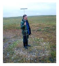
Figure 19. Anatoly Gubarkov with active-layer probe used for measuring depth to the permafrost table. Photo no. DSC\_0180, 8/27/07, D.A. Walker.
