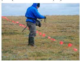
Figure 18. Howie Epstein sampling NDVI using the PSII Spectrometer. Photo no. DSC 0175, 8/23/07, D.A. Walker.
