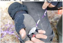
Figure 20. An iButton logger wrapped in duct tape with the logger number.
