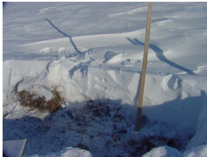
Photo 6. Snow pit at Deadhorse grid; note hard snow slab on surface with depth hoar below. Photo by M. K. Raynolds
