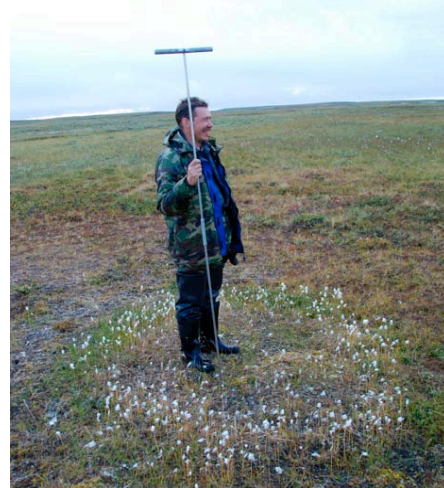
Figure 24. Anatoly Gubarkov with active-layer probe used for measuring depth to the permafrost table. Photo no. DSC_0180, 8/27/07, D.A. Walker.
