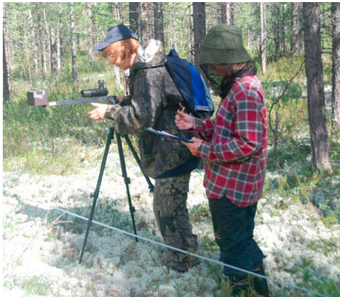
Figure 22. Buckner point-intercept sampling device. The box on the end piece of the device contains a mirror that can be pointed down to the ground or up to the forest canopy. The tube is a telescope that magnifies the image in the mirror. Cross hairs in the sighting device identify a point that intercepts a plant species which is recorded as a “hit”. The percentage cover of an individual species or cover type is the number of hits for that type divided by the total number of hits. Photo no. DSC_0151, 8/06/07, D.A. Walker.
