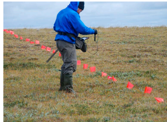
Figure 23. Howie Epstein sampling NDVI using the PSII Spectrometer. Photo no. DSC_0175, 8/23/07, D.A. Walker.
