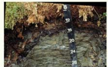
Hummock formed from frost boil due to perennial frost heave by accumulation of aggradational ice in the intermediate layer of permafrost in response to vegetation development (Coldfoot, Alaska) Scale in inches
