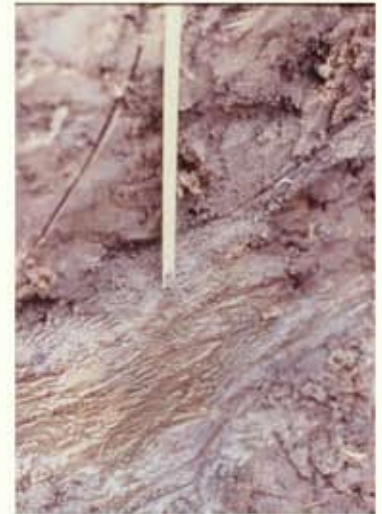
Active layer - permafrost contact in the frost boil near inter-boil area. Note orientation of ice inclusions. Barrow, Alaska
