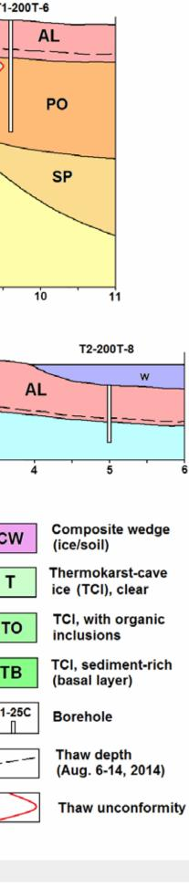
Borehole drilling encountered massive ground ice, including wedge ice (WI), thermokarst cave ice (TCI) and composite (ice/soil) wedges (CW) (Fig. 10).
